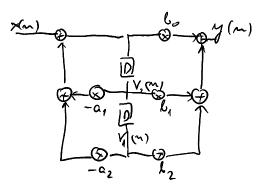
$$V_{2}(m+1) = -a_{1} V_{2}(n) - a_{2} V_{1}(n) + \times (n)$$
