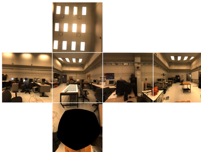
Fig. 3. Data contained in a "cube", six perpendicular perspective images are stored representing all light rays incident to a world point. This cube is one of the ones used in the experiments in this paper, it was captured from the Point Grey Ladybug camera.
