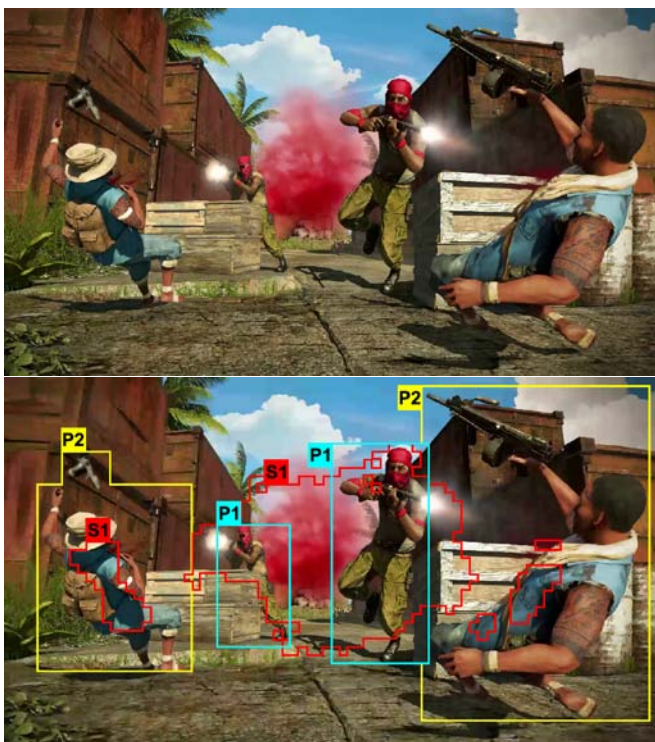
Fig. 5. A sample game frame encoded once by a single QP value (top) and another time with three QP values (bottom)
